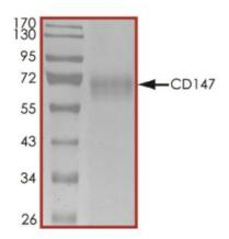
The purity of CD147 protein (REC31872) was determined to be >90% by densitometry, and MW approximately 70 kDa.
